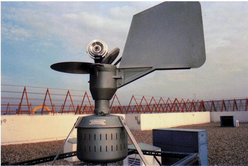
Figure 4: Sampler installed on the flat roof of the Educational Sciences Faculty, about 15 metres above ground level. Raised from the ground using a metal tower. University of Córdoba.
