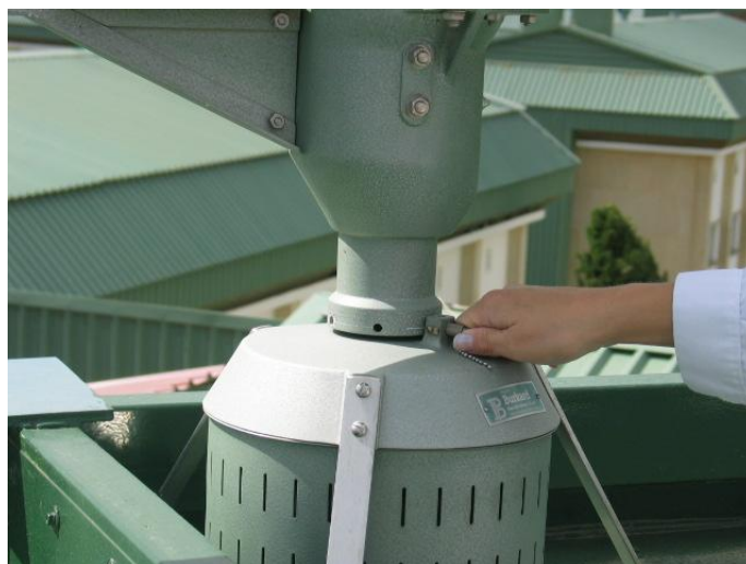
Figure 6: Securing the vane.
