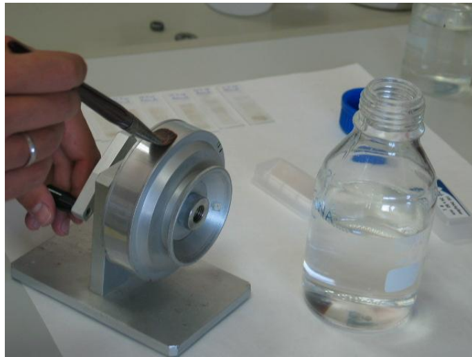
Figure 5: Application of silicone fluid to the Melinex tape wound around the drum.
