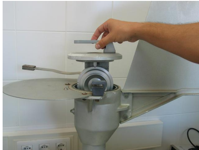
Figure 9: Placing the head inside the metal casing of the impact unit.
