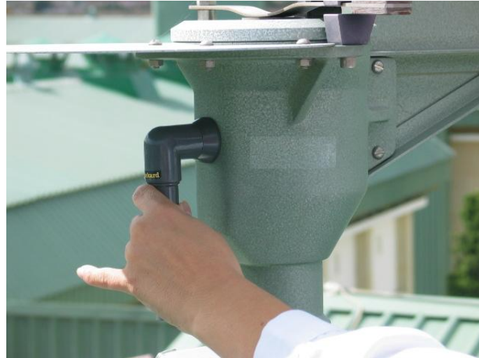
Figure 7: Checking the flow rate.
