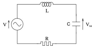
$$R = 1 \text{ K}\Omega \quad L = 100 \text{ mH} \quad C = 0.2 \text{ }\mu\text{F}$$
