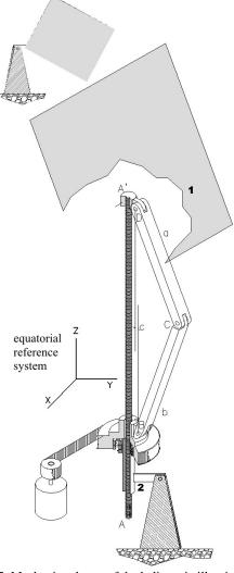
Fig.5. Mechanic scheme of the heliostatic illuminator
