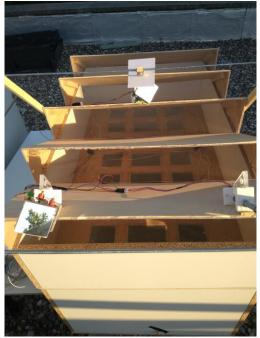
Fig.11. Layout of the 1: 15 scale models of the heliostatic illuminators on the roof of the chosen classroom of the Leonardo da Vinci building of the Campus of Rabanales at the University of Córdoba (Spain).
