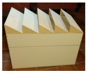
Fig.6. External appearance of the 1:15 scale model of the chosen classroom of the Leonardo da Vinci building of the Campus of Rabanales at the University of Córdoba (Spain).
