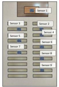
Fig.8. Layout of the TSL2561 sensors inside the 1:15 scale model of the chosen classroom of the Leonardo da Vinci building of the Campus of Rabanales at the University of Córdoba (Spain).
