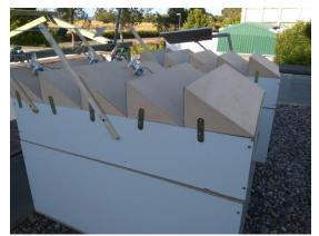
Fig.15. Measurement campaign on the 1:15 scale models of the selected classroom of the Leonardo da Vinci building of the Campus of Rabanales at the University of Córdoba (Spain).
